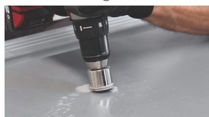
1. Round Cut with Diamond Blade Drill
