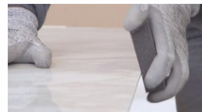
3. Refining Smooth Rough Edges With A Diamond Polishing Pad
